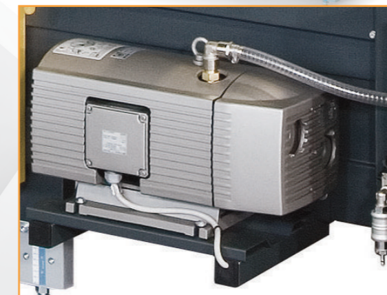
Vacuum pump for box picking
